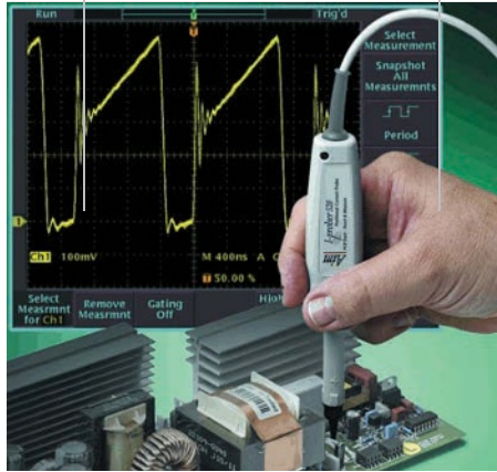
The Aim I-prober 520 positional current probe uses a patented technology to observe and measure current without breaking or surrounding the conductor.
